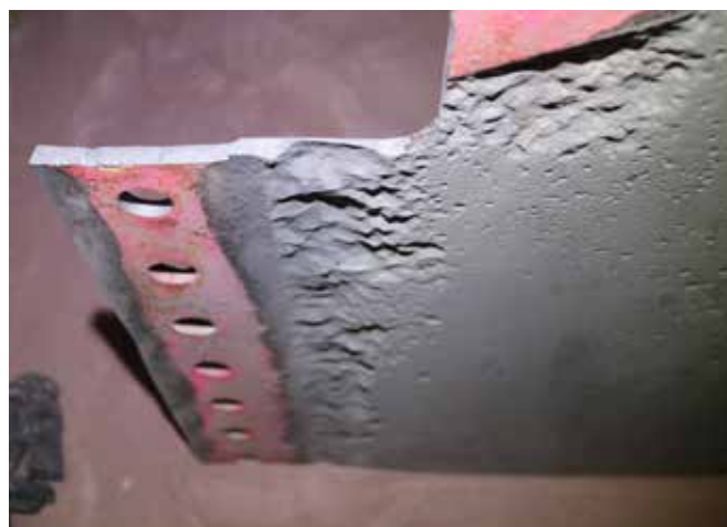
3-Way plate corrosion and pitting
